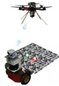
Fig. 1. UAV/UGV coordinated architecture image's bottom line. Then, the UAV can provide a vision system as a relative sensor, and fuse this information with the absolute position of the ground robot in order to achieve an absolute measurement of the position of the obstacles. By doing this, it is possible to obtain a mechanism of collaborative navigation and perform the rescue task effectively.
